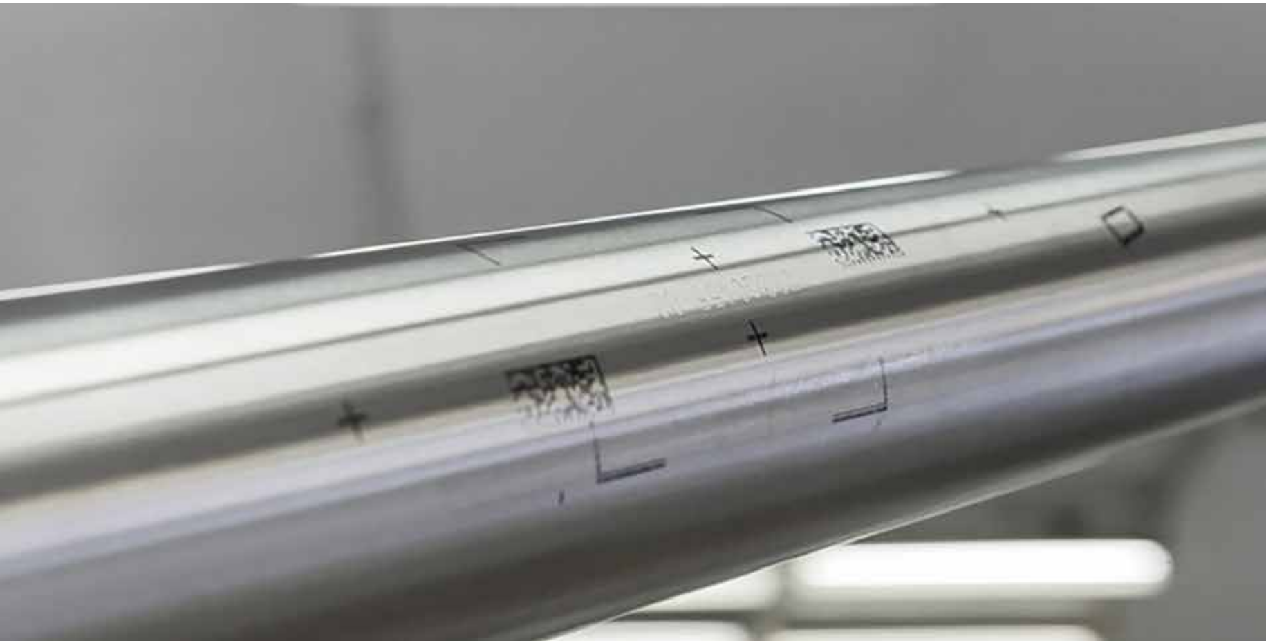
Each of the 75,000 steel tubes has a unique QR/serial code identifying its exact location on the building.
